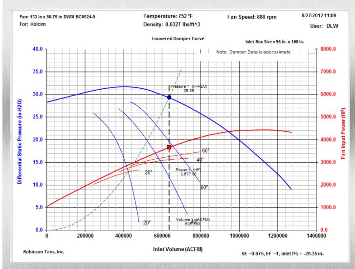
The actual operating point will be the intersection of the system resistance curve and the fan curve.
