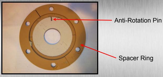
Seal assembly shown from fan side
