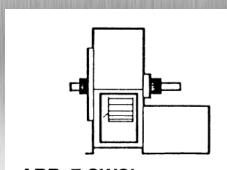
**ARR. 7 SWSI**For belt drive or direct connection. Arrangement 3 plus base for prime mover.
